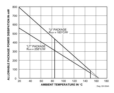
NOTE – Permitted duty cycle will be less than 100% at maximum ambient temperature with high supply voltages, i.e.,  $T_A \oplus 140^{\circ}\text{C}$ ,  $V_{CC} \oplus 12 \text{ V}$ , and the "LT" package. The thermal shutdown circuitry does not protect the device from these stresses (see Internal Protective Features).
