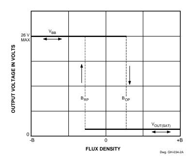
**Power Up Reset.** These devices are designed to power up with the output OFF without regard to any magnetic field applied. The output will remain OFF until the flux is reduced to below  $B_{RP}$  (S-N transition) and then  $B_{OP}$  is exceeded, depending on the turn-on state of the internal latches.
