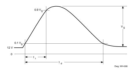
Power supply voltage transients, or device output short circuits, may be caused by faulty connectors, crimped wiring harnesses, or service errors. To prevent catastrophic failure, internal protection against overvoltage, reverse voltage, output overloads, and thermal stress have been incorporated to meet the automotive 12 volt system protection requirements of ISO DP7637/1 and DIN 40839-1. A seriesblocking diode or current-limiting resistor is required in order to survive pulse number six.
